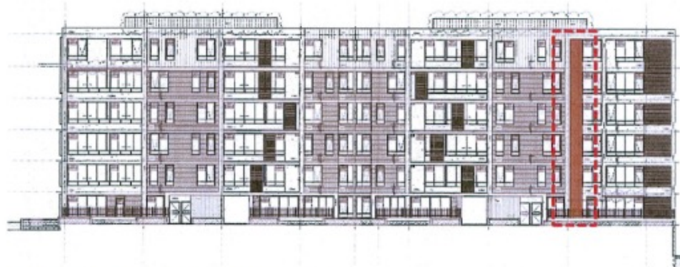
Figure 8: Southern Elevation of Building 1 – Biowood cladding
